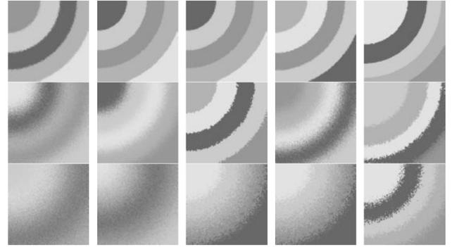
Fig. 3. Visualized clustering results on images from Fig. 2: original images(first row), images corrupted by noise ratio of 5% (second row) and images corrupted by noise ratio of 10% (third row), respectively by: FCM (first column), sFCM (second column), gFCM (third column), bFCM (fourth column) and wFCM (fifth column)
